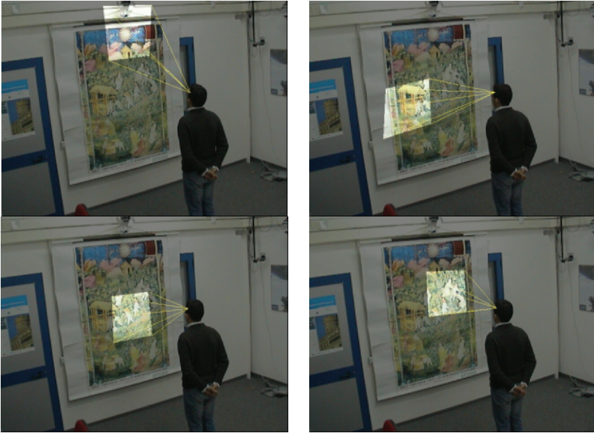
Fig. 15. Real time head orientation can support contextualized information delivery in museum environments. The highlighted areas on the picture represent the projection of the user viewing frustum onto the exhibit as determined automatically by the system. The user could be given audio feedback by means of wireless earphones
