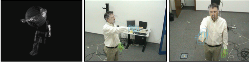
Fig. 16. Left: Elliptical linkage test arcs used to associate hands to heads. Right: Clustering head and hand skin hypothesis represented as voxels in 3D space provides more robust results
