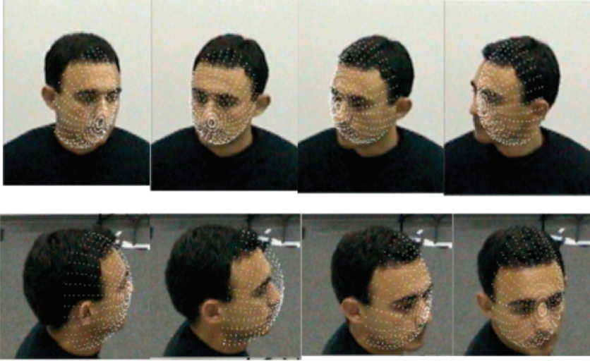
Fig. 14. The performance of the pose estimation tracking algorithm on a real sequence captured from two different cameras
