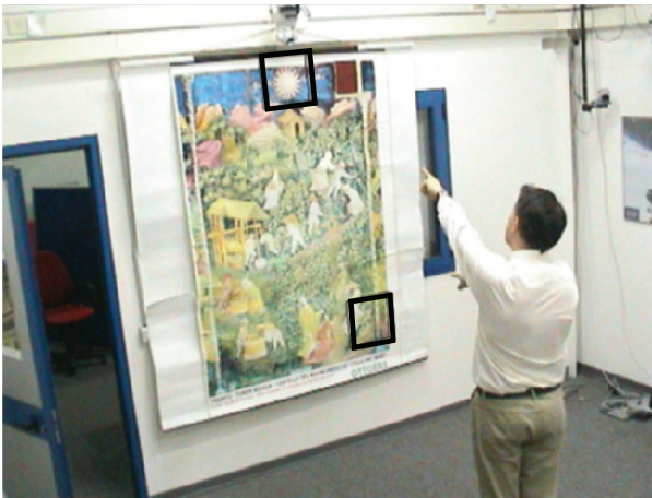
Fig. 18. Two hands used to links different parts of the exhibit. Assuming that each hot spot (boxes) on the painting is given a numerical index i , a two-hand gesture like the one detected in the picture may be used to address an element in a two-dimensional matrix M_{ij} . Each such element may be associated to a multimedia presentation that provides in depth information on the relation between the two selected hot spots
